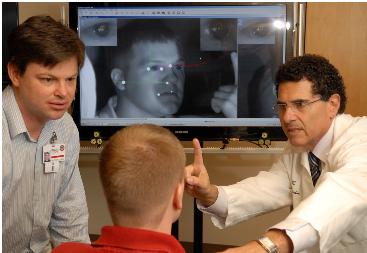
Caption: Dr. Randy Kardon is one investigator funded through the Peer Reviewed Vision Research Program. Here, Kardon (right) and researcher Pieter Poolman (left) work on a new system that uses four separate cameras to simultaneously track head, eye and pupil movements in order to determine how accurately a patient's eyes track targets.
